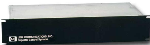
The Atlanta Radio Club's Link Communications RLC-3 is just such a controller. From high atop the Bank of America building, it controls the 146.82, 224.34 and 444.825 repeaters as well as an autopatch and links to IRLP, Georgia Skywarn, The Southeastern Linked Repeater Net and several remote receivers for the 2-meter system.
